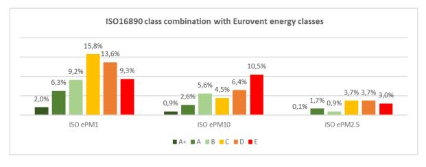
Figure 6. ISO Class rating acc. to EN ISO16890: 2016 and Eurovent energy efficiency class percentage
