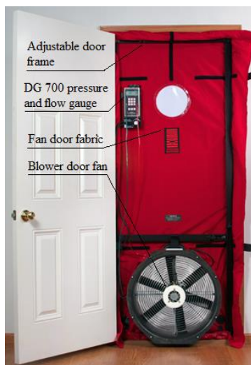
Figure 2. Standard Minneapolis blower door unit (photo source: Wikimedia )
